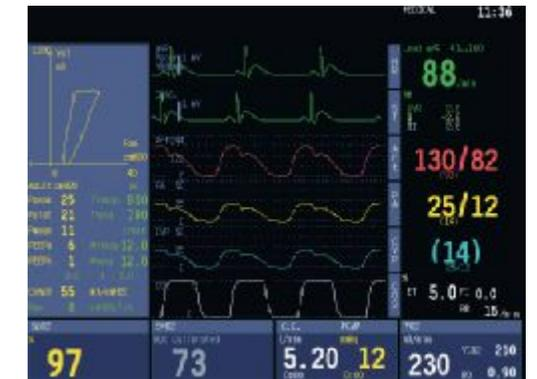
**Spirometry split screen** enables real-time monitoring of spirometry loops and numerical values, combined with hemodynamic information or real-time waveforms of airway pressure, flow and gases.
