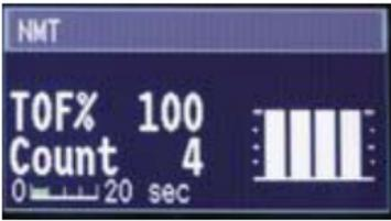
1. Attach MechanoSensor to the patient's hand with tape. The monitor will start measurement by setting the stimulus current automatically and by performing a reference measurement. With the unrelaxed patient, TOF% is 100.
