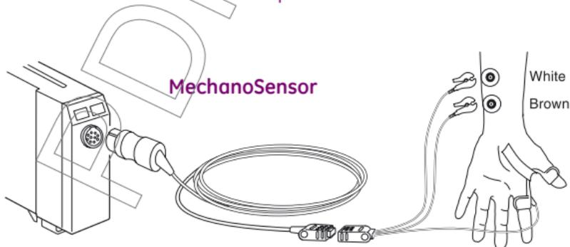
*NMT measurement setup with MechanoSensor.*
