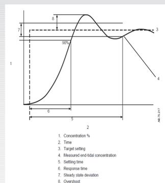
**Fig 3. Variables used for analysis of gas setting change (concentrations measured from the patient's airway)**
